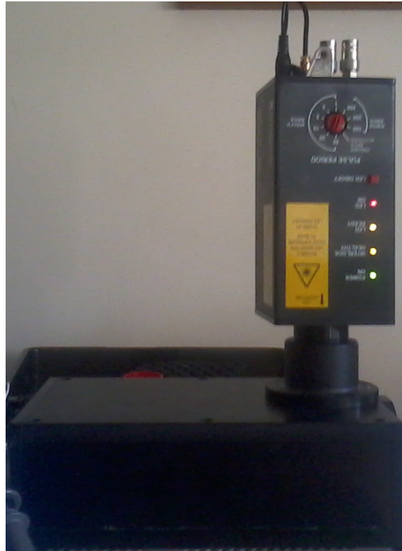
Figure 5.1. Box containing the photodiode array and the pulsed led.
