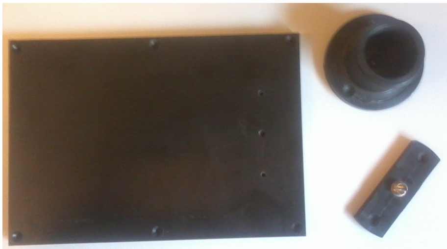
Figure 6.1. Picture of the hole made into the top side of the box and its dedicated adapters.
